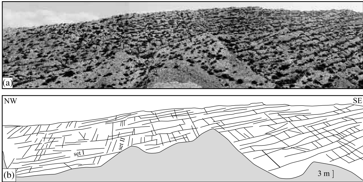
Fig. 11. Fracture pattern in the backlimb. (a) Field photograph at site 8 in the Tensleep sandstone. (b) Line drawing of the outcrop in (a) that shows Set II fractures (strike of 045^\circ ) terminating at Set I fractures (strike of 110^\circ ).
